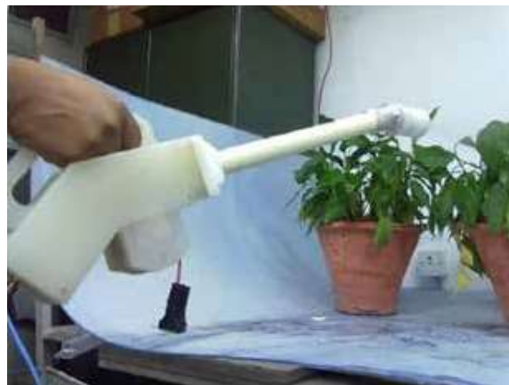
Figure 60 An Electrostatic Nozzle
