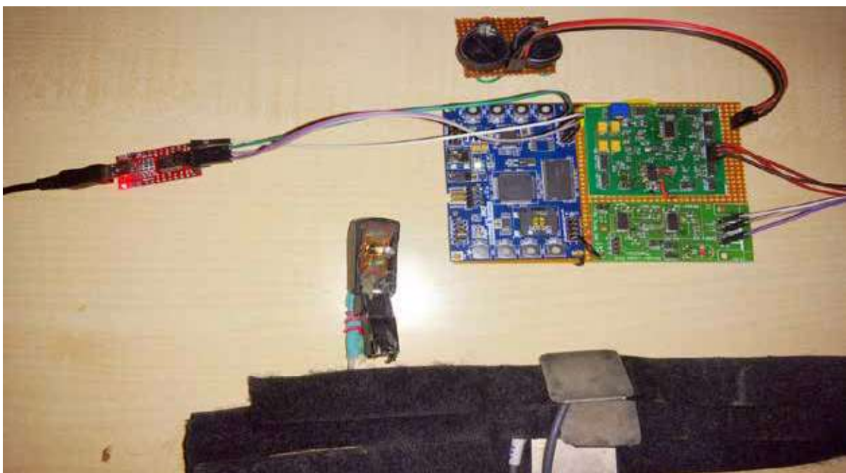
Figure 71 Preliminary hardware prototype for cuff less BP monitoring
