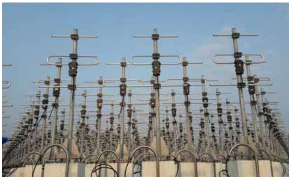
Figure 61 The 619 element antenna arrangement of ST radar
